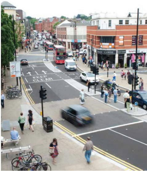
Wide crossing points at key routes indicated with raised tables and a change in surface materials. Wimbledon station (left) and The Strand (right) (Better Streets Delivered, Transport for London 2013)
