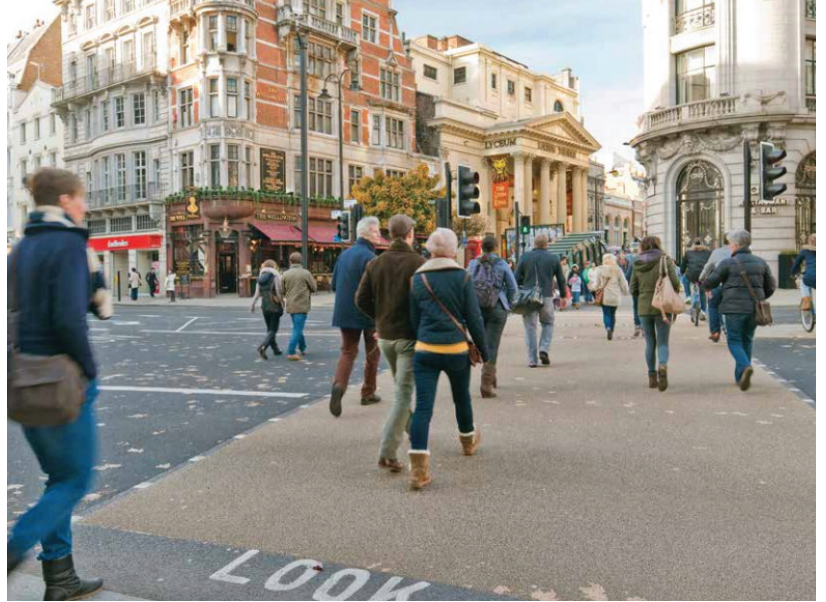
Wide crossing points at key routes indicated with raised tables and a change in surface materials. Wimbledon station (left) and The Strand (right) (Better Streets Delivered, Transport for London 2013)
